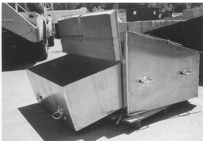
FIGURE 1. The box-type solar cooker was tested by the U.S. Forest Service and the U.S. Park Service to pasteurize the end-product from public composting toilets used by hikers in the backcountry. Photographs by Paul Lachapelle.
