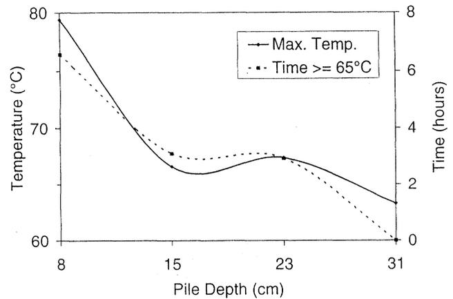
FIGURE 5. Comparisons are made between pile depths, the maximum temperature attained, and the duration in hours at or above  $65^\circ\text{C}$ . Moisture content of the compost pile is equal (33.5%). Temperature readings are taken from the middle of the compost pile.
