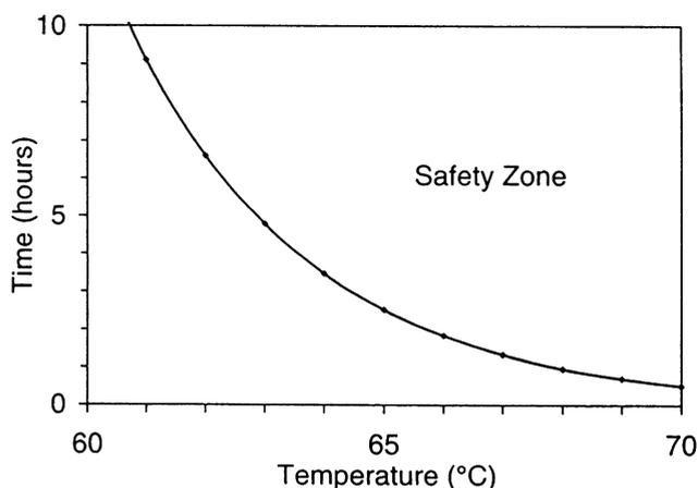
FIGURE 2. U.S. Environmental Protection Agency (EPA) 40 Code of Federal Regulations (CFR) Part 503, time-temperature relationship for the heat-treatment of sewage sludge.
