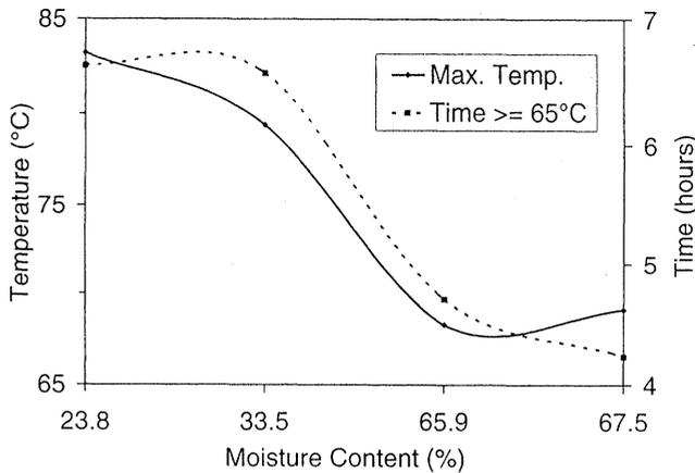
FIGURE 4. Comparisons are made between percentages of moisture content, the maximum temperature attained, and the duration in hours at or above  $65^\circ\text{C}$ . All pile depths are equal (8 cm). Temperature readings are taken from the middle of the compost pile.
