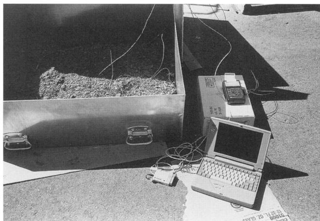
FIGURE 3. Two time-temperature data loggers were used to record and compare temperatures within the Hot Box. Temperature probes were inserted into various sections of the compost pile through a small hole in the back of the Hot Box. A laptop computer was used to download and display the data from the data loggers. Photograph by Paul Lachapelle.
